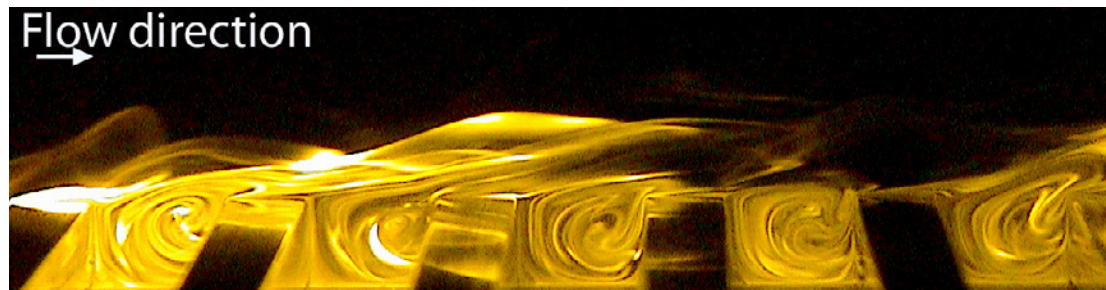
a) Skimming flow visualization for gap distance s/k = 1.5 between slats
